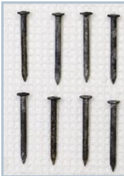
G90 Galvanized Nails Installed in ACQ Lumber After 4 months Humidity Testing
