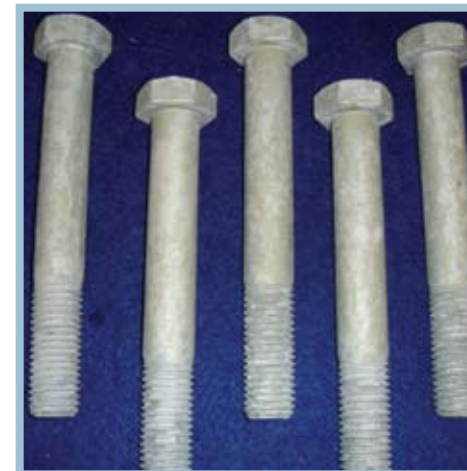
3/4" Bolts Magni Coatings 1000 hours of ASTM B117 testing
