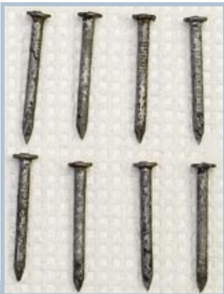
Magni 599 Coated Nails Installed in ACQ Lumber After 4 months Humidity Testing
