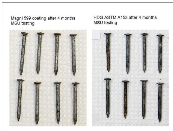
Figure 3 - Magni 599-coated nails compared to HDG nails after 2880 hours in MSU/Osmose corrosion test
