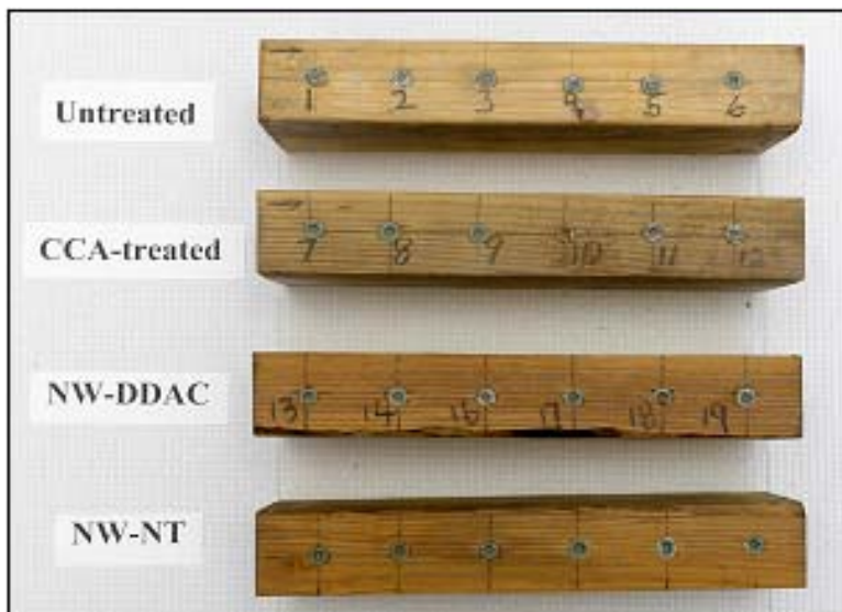
Figure 1 - Magni 599 after 2160 hours in MSU/Osmose corrosion test
