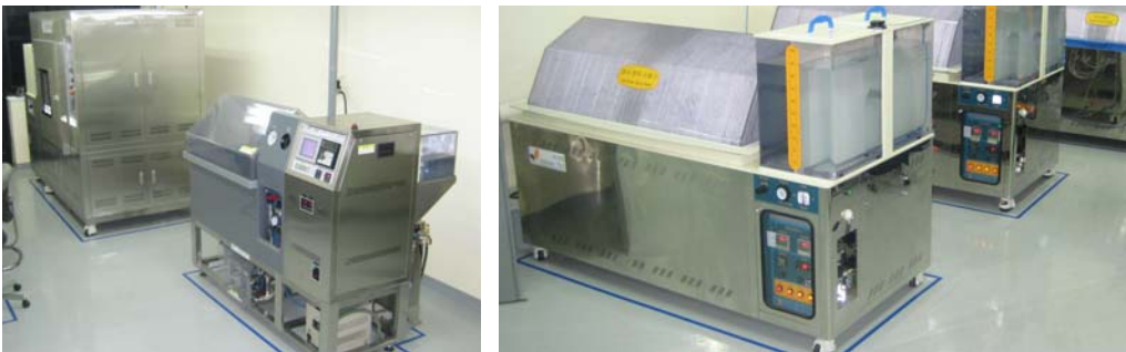
Cyclic Corrosion Test Cabinets (GM Dat & Hyundai) and Salt Spray Test Boxes 8/25/08
