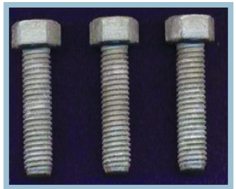
Magni 565 at 1,000 Hours ASTM B117
