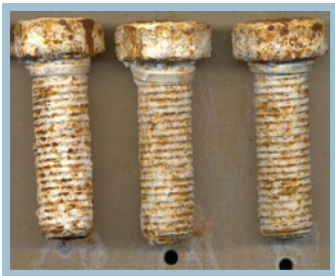
HDG at 500 Hours ASTM B117
